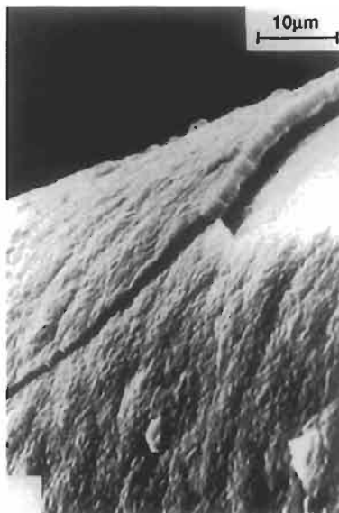
Fig. 5.25. A scanning electron microphotograph of fractured yttria coating on a SiC monofilament after cooling through 500°K. After Kiescheke et al. (1991a). Reproduced by permission of Elsevier Science Ltd.
